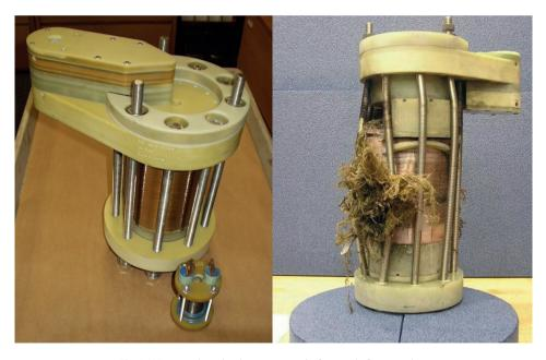
The LANL 80 tesla pulsed test magnet before and after 10 pulses
