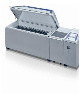
A precision two-component nozzle ensures optimal spray mist distribution. The two material nozzles are used to nebulise the salt solution in the testing chamber. These are arranged in specialised spraying channels in the walls of the chambers.
