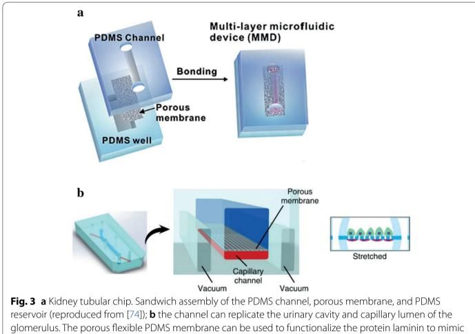
glomerulus. The porous flexible PDMS membrane can be used to functionalize the protein faminin to mimic the glomerular basement membrane. Cyclic mechanical pressure to the cell layer via vacuum stretching of the flexible PDMS film can be produced (reprinted with permission from [76] Copyright © 2018, Royal Society of Chemistry)
