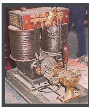
*DC* machine and the brush gear position had to be advanced or retarded by hand to suit the load conditions.
