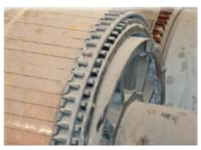
3. Double Cage Bar Wound Motor Rotor.
