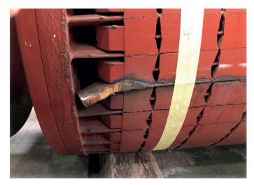
10. Rotor bar fractured and lifted damaging the stator winding.
