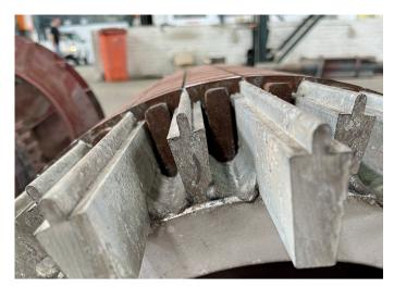
5. Aluminium Rotor bars brassed to Aluminium end rings.
