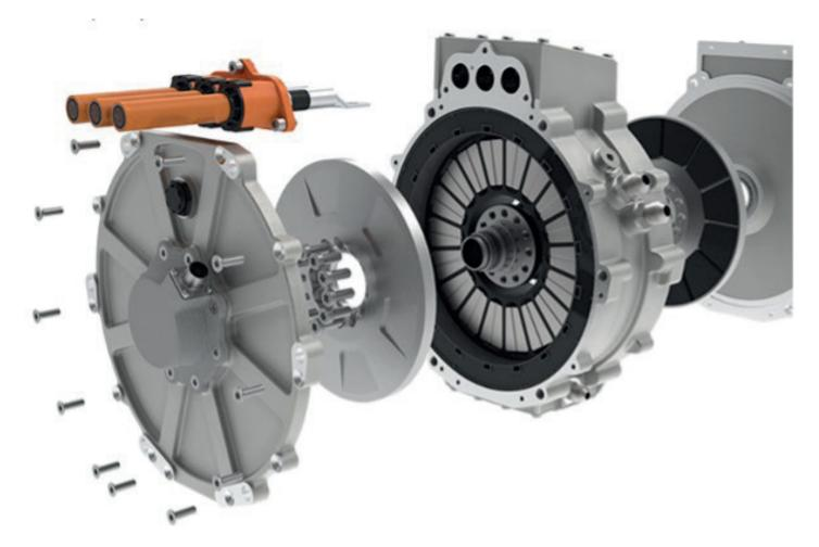
Exploded view of an axial flux motor showing 18 electromagnet stator cores mounted in housing and two permanent magnet carrying rotors which can be bolted to the shaft. Note the 3-phase connecting box at top of housing and cooling air connections at side.
