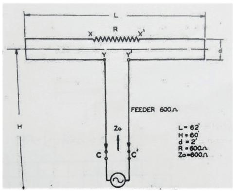
Figure 8: The resistively-loaded folded dipole antenna
