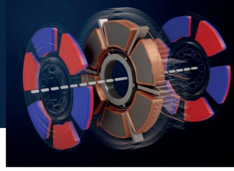
Axial flux motor components - The rotors with permanent magnets will usually be fixed to the shaft, and the stator with windings fixed to the housing The hinted ball bearings in this illustration indicate a direct drive vehicle motor with rotating housing and power supply through the stationary shaft.
