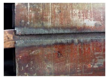
9. Rotor Lamination Core burning due to fracture bar.
