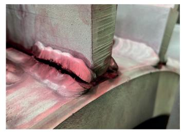
7. Aluminium Bar welding Failure.
