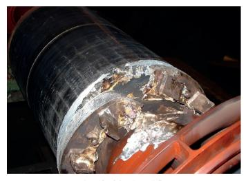
8. Cast Aluminium Rotor Failure.
