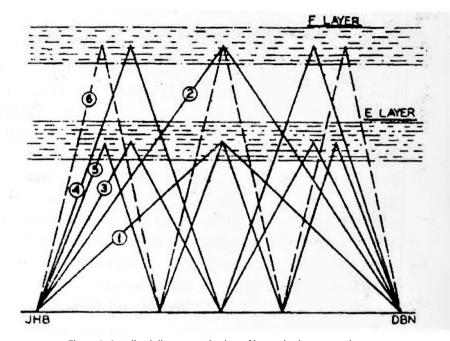
Figure 9: A stylised diagrammatic view of ionospheric propagation.
