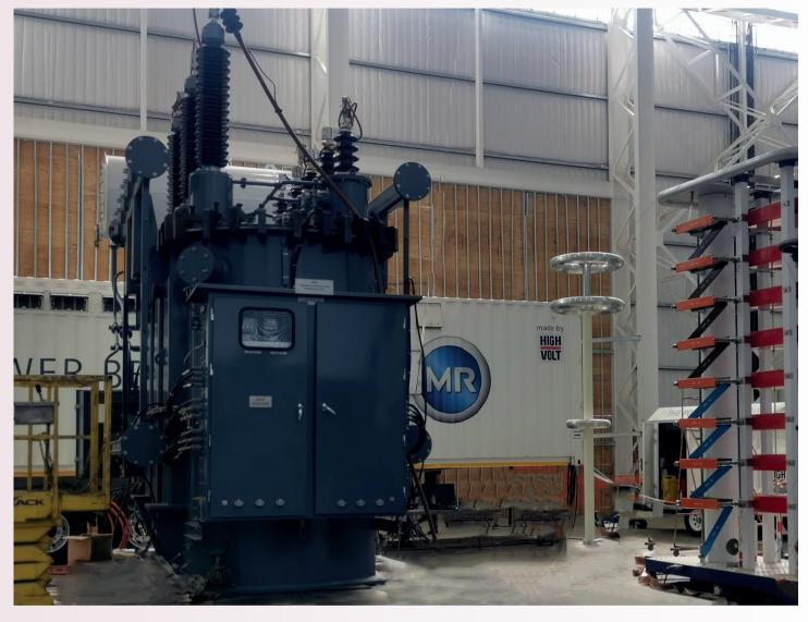
SGB-SMIT POWER MATLA is proud to celebrate a significant milestone marking the commissioning and operation of the on-site testing facility since the fire accident at the Pretoria power manufacturing plant in March 2021. In the newly built on-site test facility, the team successfully manufactured and tested a 45MVA 88/11kV double-wound three-phase transformer manufactured for a local utility on 8 March 2022.
