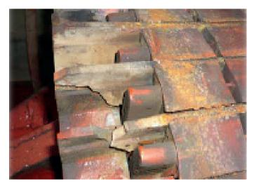
6. Cage Bar Wound Induction Motor Rotor Failure.
