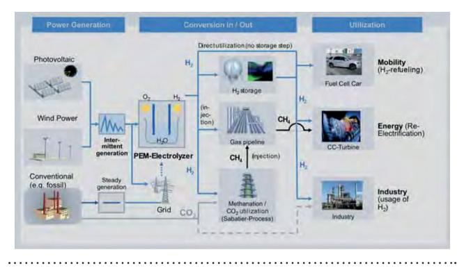
Figure 2-8 | Overall concept for the use of hydrogen and SNG as energy carriers [wai11]
