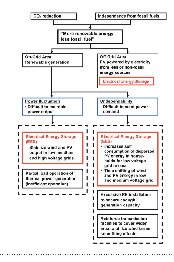
Figure 1-2 | Problems in renewable energy installation and possible solutions (TEPCO)
