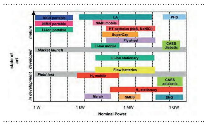
Figure 2-11 | Maturity and state of the art of storage systems for electrical energy (Fraunhofer ISE)
