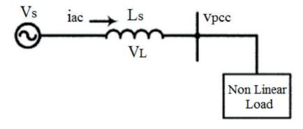
load currents. Thus, in principle, end users and utilities share responsibility for limiting harmonic current injections and voltage distortion at PCC. Since there are two parties involved in limiting harmonic distortions, evaluation of harmonic distortion is divided into two parts measurements of the currents being injected by load and calculations of frequency response of system impedance.
