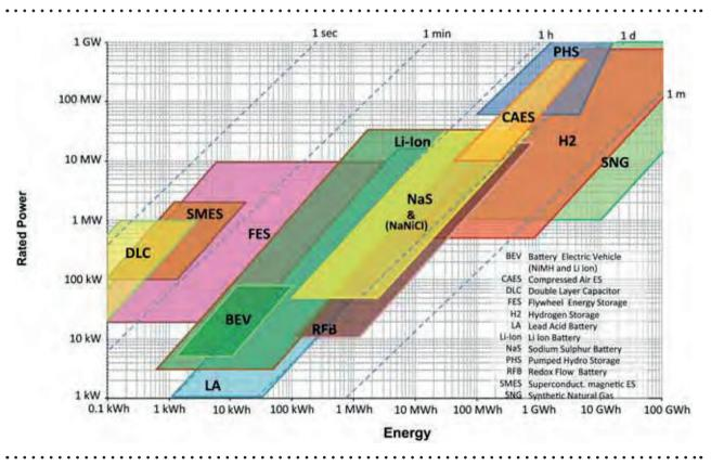
**Figure 2-9 | Comparison of rated power, energy content and discharge time of different EES technologies** (*Fraunhofer ISE*)
