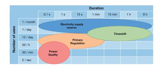
Figure 1-3 | Different uses of electrical energy storage in grids, depending on the frequency and duration of use [eus06]
