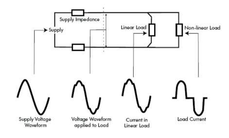
Voltage Distortion - Close Coupling
