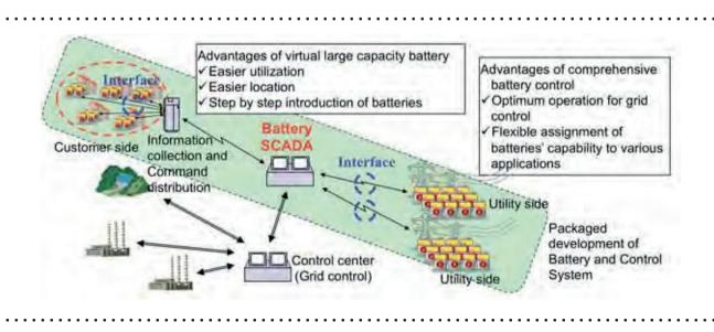
Figure 3-20 | Schematic diagram of Battery SCADA (TEPCO)
