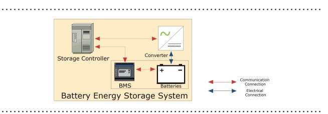
**Figure 3-17 | A possible realization of internal control architecture for a battery storage system** (*ABB*)
