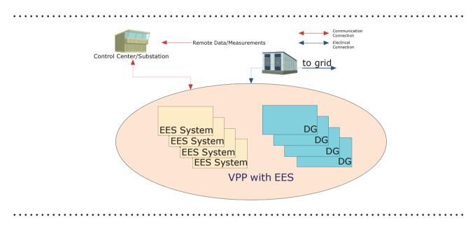
Figure 3-19 | A generalized control concept for aggregated EES systems and DGs (ABB)
