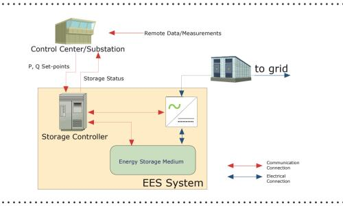
Figure 3-18 | A Control hierarchy involving remote data/measurements (ABB)
