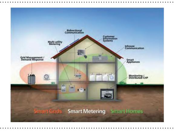
Figure 3-14 | The Smart House (Fraunhofer ISE)
