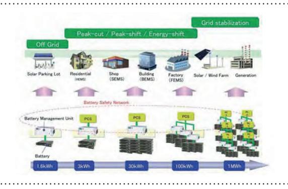
**Figure 3-13 | Scalable architecture for EES applications in a Smart Microgrid** (Sanyo, IEC MSB/EES Workshop, 2011)
