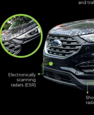
The Ford Edge-based test vehicle is equipped with Level 3 autonomous capabilities on an open-source platform – differentiated from other test vehicles that either only test within closed courses or are limited to a host company's proprietary platform.
