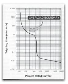
Figure 2c Overload boundary of typical item of electrical equipment
