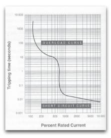
Figure 2d Typical tripping curve for an MCCB
