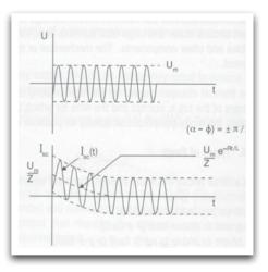
Figure 2b Asymmetrical short circuit condition
