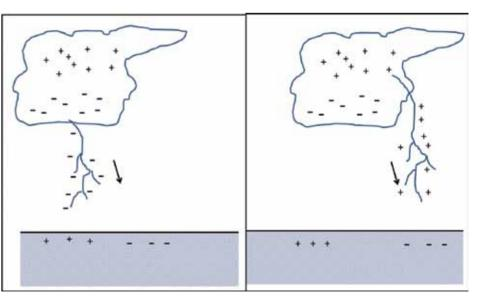
Figure 6: The main types of *lightning flash [1].*
