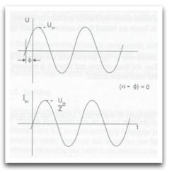
Figure 2a Symmetrical short circuit condition
