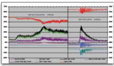
Figure 3: Shredder Operating Modes with and without Power Correction
