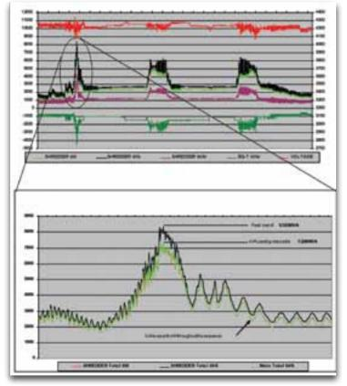
Figure 4: Record Metal Shredder Power Consumption (Bottom Graph is an Enlarged View of this Event)
