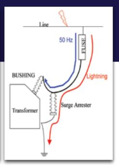
*Fig 6. Incorrect placement of the surge arrestor at the pole-mounted transformer.*
