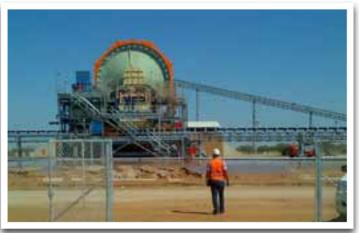
The fully autogenous grinding mill at Boteti powered by a WEG solution comprising a 4 000 kW 3.3 kV motor, a MVW01 VSD and phase shift transformer.
