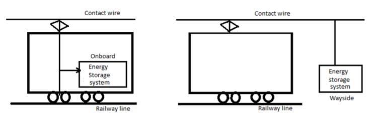
Figure 4a: Illustration of onboard ESS
