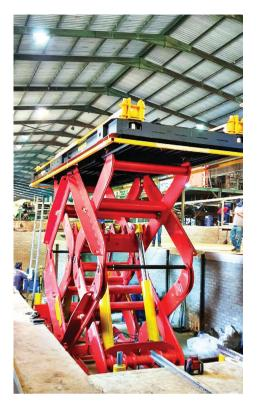
Up and coming dock-levelling manufacturer, REV Designs, recently completed the design and construction of three of the country's largest scissor lifts ever produced with a capacity of up to 40 tons per lift.
