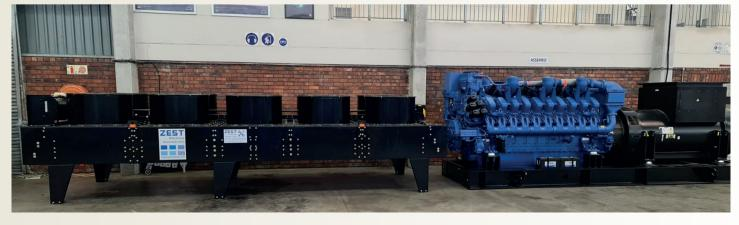
Table top radiator with diesel engine coupled to WEG alternator.
