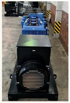
The WEG MV alternator, in front, coupled to the diesel engine.
