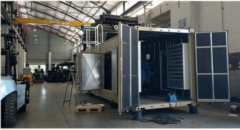
During fitment of the engine and alternator within the generator enclosure at Zest WEG's local manufacturing facility.
