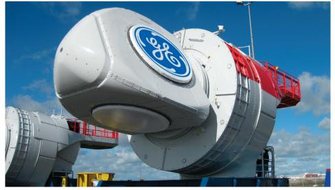
GE Haliade-X direct-drive permanent magnet alternator and nacelle
