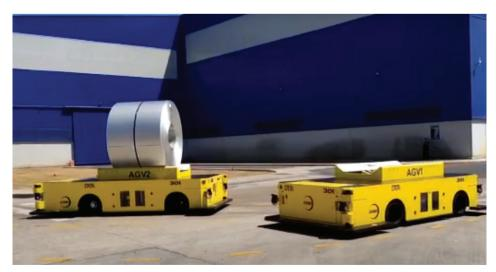
The two AGV's in Acerinox Europa crossing at an intersection one with a 30 ton stainless steel coil payload.
