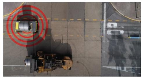
Safety sensors continuously scan for obstacles. If detected the vehicle automatically stops.
