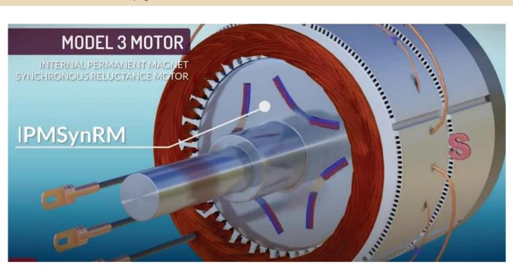
Tesla vehicle reluctance motor with neodymium magnets embedded in the rotor
