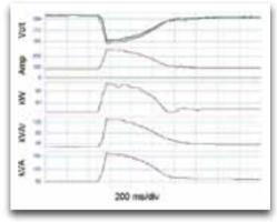
Figure 6: Typical dip at MCC
