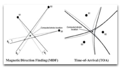
Figure 1. Locating lightning strokes with Magnetic Direction Finding and Time-of-Arrival techniques.
