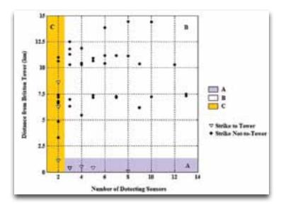
There are two measures of how effectively an LDN is operating: Detection Efficiency and Location Accuracy.
