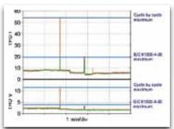
Figure 9: Cycle-by-cycle and IEC 61000-40-30 THD
