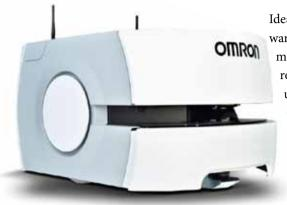
Ideal for conveying goods throughout warehouses, distribution centres, and manufacturing facilities, the LD mobile robot platform has a payload capacity of up to 130 kg, depending on the model. Compared to traditional Automated Guided Vehicles (AGVs), Omron mobile robots can self-navigate entirely based on the natural features of the facility.
