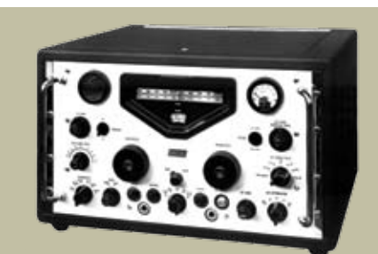
Trevor Wadley's radio receiver design was used in the Racal RA117, seen above.
