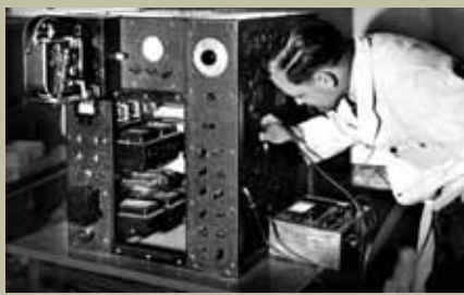
Wadley inspecting Ionospheric Recorder with a continuous coverage from 0,1 – 2 MHz.
