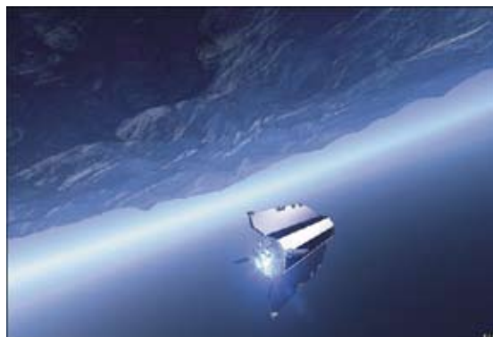
Goce aims to map Earth's gravity field to an accuracy of one mGal (about a millionth of the acceleration due to Earth's gravity at its surface). It expects to determine the geoid to a precision of one to 2cm and achieve this at resolutions down to 100km.
