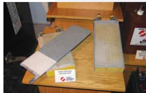
Deep cycle batteries are designed to be charged and discharged every day. To prevent shedding of active material, the positive plates are constructed with a row of spines each enclosed by their own individual tube.
