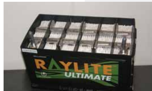
The Raylite Ultimate is a valve regulated lead acid (VRLA) battery that uses absorbent glass mat (AGM). The battery is built under high compression, 25 kPa, to hold the AGM in contact with the plates and prevent shedding. The result is both a higher power density and better cycling characteristics.
