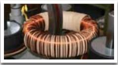
Copper Wire Being Wound Onto The Core
