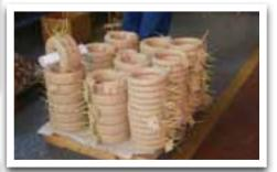
*Testing Of Secondary Coils* The winding ratio of each Secondary coil is tested for turn accuracy. This is done by injecting the full load current (1000A 1200A etc) through the coil, and measuring the output.
