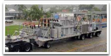
A WEG 30 MVA 138/69 34.5/13.8 kV mobile substation with an hydraulic goose neck and articulated rear wheels to accommodate tough terrain and any logistic challenge.
