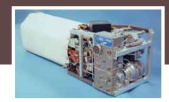
Figure 10 – Space Shuttle fuel cell. The shuttle employed three of these. [Source: NASA]
