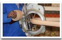
Insulating tape being wrapped onto copper
