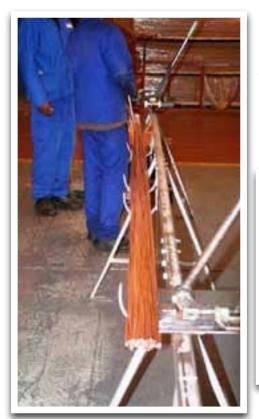
Solid copper conductors wrapped together
