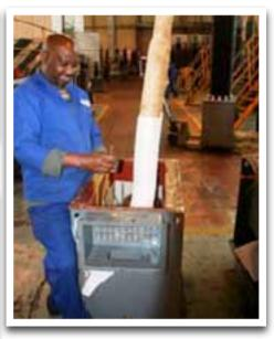
When fully assembled the complete current transformer is placed into the secondary oven and dried.
