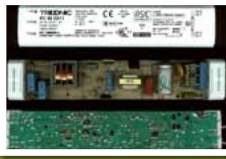
Figure 2: Interior of an electronic ballast – it inverts the mains frequency into high frequency, which allows for building the inductive components substantially smaller and eases the inclusion of electronic control
