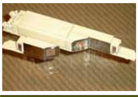
Figure 1: Interior of a magnetic ballast – nothing much more than an iron core and a copper winding in there
